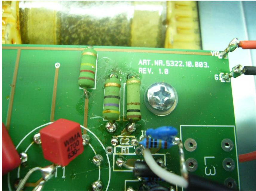
*These resistors can also be burned by a bad power tube but are more robust than the trim pot.*
