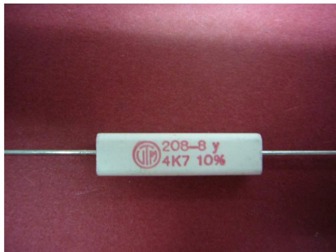
*Please solder this new resistor with a bit distance from the board of the generated heat of this component. The extra space from the board will aid in heat dissipation. For procedure see "Replacing Components".*
