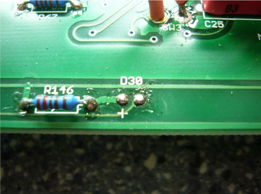
*The + mark on the board should be connected to the long pin on the LED:*
