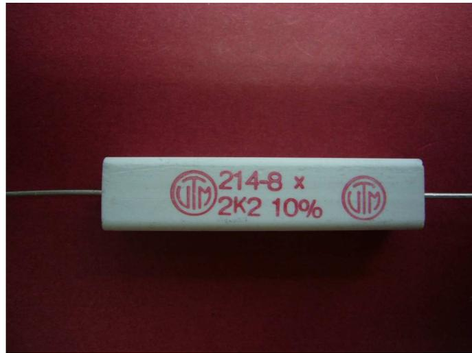
*Replace this resistor with a 4,7k ohm / 5 watt type:*
