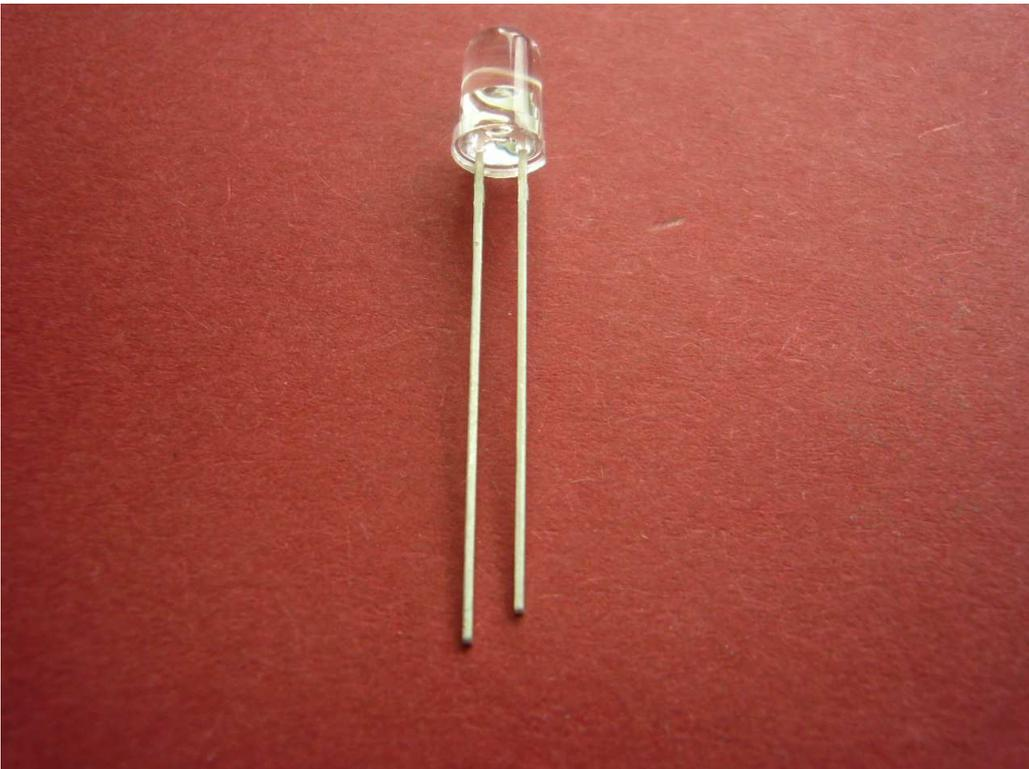
*Shorten the pins on the LED a bit for good fit, and solder the LED to the board. Bend the leads to get the LED through the hole in the front panel. Be sure that both leads do not touch or are shorted by an insertion tool:*
