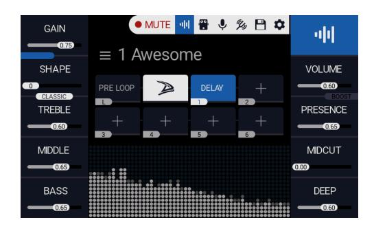
The UPPER section displays the current PRESET, so **PRESET NUMBER** from 1 to 99 and **PRESET NAME**.
