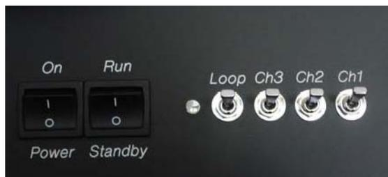
On the left of the pots are the switches for the channels and the loop on/off switch. Each switch also has an LED indicator, the loop LED on the left of the switch, the channel's LED are located between the pots of each channel.
