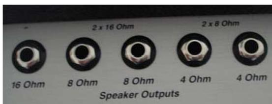
**WARNING:** Although the Schmidt amplifier has 5 speaker outputs never attempt to connect more speakers than rated. The safe combinations are 1x16 Ohm, 1x8 Ohm, 1x4 Ohm, 2x16 Ohm or 2x8 Ohm. Any other speaker configuration may stress the power amplifier section and in extreme cases may lead to valve and/or output transformer failure.
